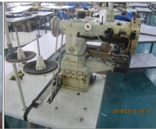
Photo of non-conformity sewing machine missed the pulley guard.JPG
